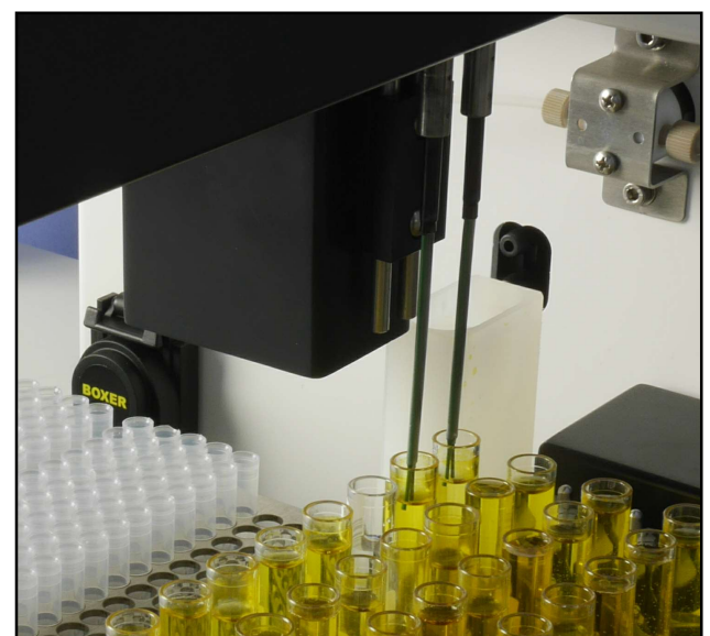
Dual nozzle probe aspirating sample
