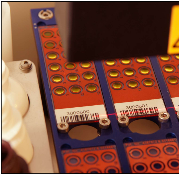
Linear barcode reader acquiring barcodes from slides
